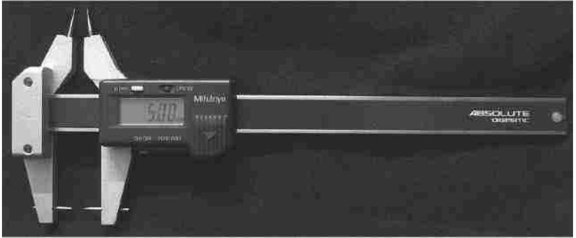
Fig. 5.6. The Hillson-Fitzgerald calliper for taking cervical dental measurements. Source: Hillson et al., (2005)
